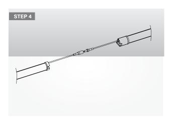
**STEP 4:** For linkable connect, just plug the female and male connector from each fixture;
