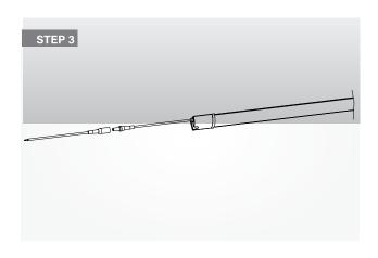
**STEP 3:** Connect the AC input wire to the one side connector of the fixture
