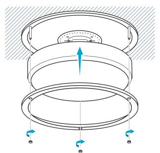
**STEP 4:** Place the plastic lens back up into place between the three pins. Align the holes in the metal ring with the three pins and use your hand to screw the decorative nuts up to the metal ring to secure the lens and ring in place.
