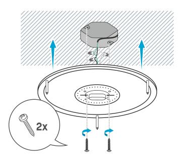
**STEP 3:** Raise fixture up to the junction box and use a screwdriver to attach the fixture using the 2 screws (provided).
