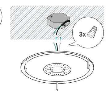
**STEP 2:** Connect the fixture with cables from junction box using 3 wire nuts (provided): black to black wire, white to white wire, and green / yellow to green / yellow wire.
