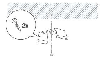
**STEP 5:** Affix the mounting brackets to the ceiling/wall. Tip: Use fixture to mark hole position.
