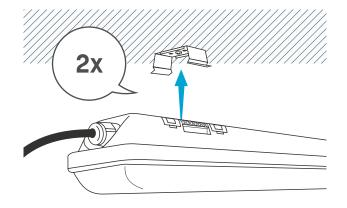
STEP 6: Affix the fixture to the ceiling/wall with mounting brackets as shown.
