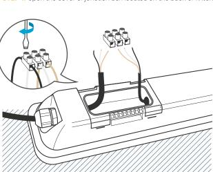
**STEP 3:** Connect the fixture with cables from junction box using the wire block connector inside the unit's junction box: black to black wire, white to white wire and yellow/green to yellow/green wire.
