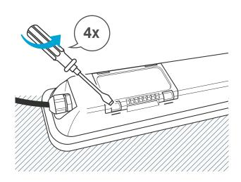
STEP 1: Open the cover of junction box located on the back of fixture.
