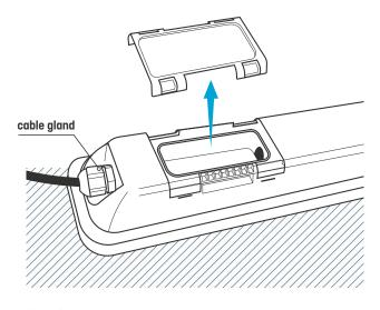
STEP 2: Insert a power cord through the waterproof 'cable gland' at the end of the unit.
