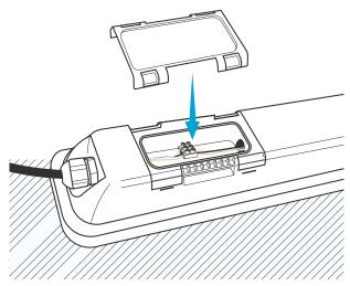
STEP 4: Close the cover back onto the fixture junction box to seal securely.
