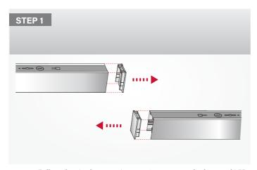
STEP 1: Follow the single mounting step1 to remove the lens and LED module, then follow the label indication to set up the CCT and power by adjusting the two switches , remove all the end caps of the fixture;
