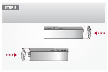
STEP 8: Assemble the end caps back on the left and right side;
