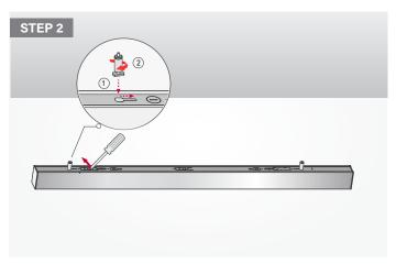
STEP 2: Put the hanging wire holder hook thru the knock out hole of the fixture, then use screw driver open the knockout hole for cable connection;
