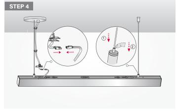
STEP 4: Put the two aircraft wires thru the wire holder of the ceiling box and ceiling until it's locked, then holdup the fixture hanging on the ceiling by inserting aircraft wire thru the wire holder on the back of fixture, pull out the connector from the big knockput hole on the back of the fixture, connect the cable from ceiling box to the fixture by plugging quick connectors;
