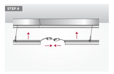
STEP 6: The assemble back the LED module and connect the cable between fixture with connector on the LED module one by one into the casing;
