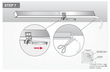
STEP 7: Assemble the lens from one end to another, then cut off the lens evenly;
