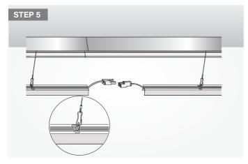
STEP 5: Hook the safety wire of the casing with the LED module
