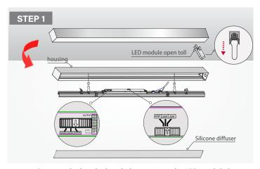
STEP 1: Remove the lens by hand, then remove the LED module by inserting and lifting up the two U-shaped clips (provided); follow the label indications to select desired color and power by sliding the two switches, then assemble the LED module and diffuser;
