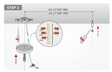
STEP 3: Install the bracket on the Jbox in the ceiling, then pull the cable thru the canopy; tighten the cable holder, make wire connections as diagram indicates. then use the screw pipe install to hold the canopy in place, mount the aircraft wire holder on the ceiling then following the instruction distance;
