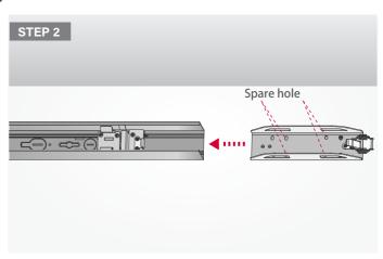
STEP 2: Plug in the insert bracket into the fixture casing end, install two screws to lock the insert;
