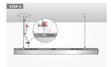
STEP 5: Put the cable cover back then assemble the screw, adjust the hanging height of fixture by pulling the aircraft wire to lift the fixture up,or push the wire holder top to release aircraft to let fixture slide down to desired height, then use the cable and aircraft holder lock together of the cable and wire;
