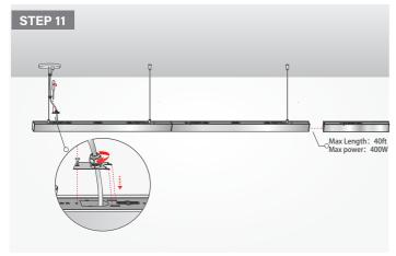
STEP 11: Put the cable cover back then assemble the screw, adjust the hanging height of fixture by pulling the aircraft wire to lift the fixture up, or push the wire holder top heard to release aircraft let fixture down, then use the cable and aircraft holder lock together of the cable and wire.
