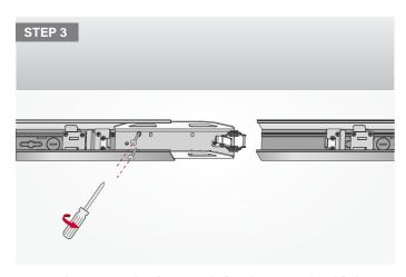
STEP 3: Plug into another fixture end after alignment, then lift the spring hook on the fixture;
