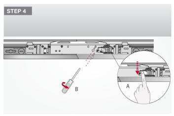
STEP 4A: Push down the spring handle until it's locked tightly;
